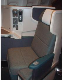
RIGHT: The latchable side cabinet can be used to store wallets, passports, phones, etc, and it also acts as the divider for privacy when left in the open position (once the aircraft is in flight).
