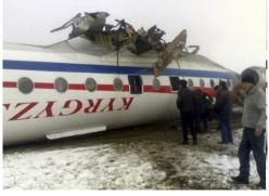
According to the Aviation Herald the plane hit the tarmac so hard as it landed that the right main landing gear collapsed - causing the wing to fall off and allowing the aircraft to roll onto its roof, as pictured above.
