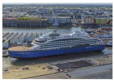
**PONANT'S** Le Commandant-Charcot (pictured) has entered the final stages of construction, arriving in Saint-Nazaire to be fitted with Azipod propulsion systems.
